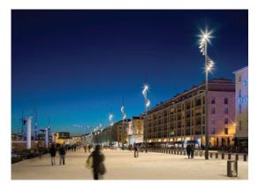
Seventeen 16.5 metre and eight 23.5 metre high custom designed Olivio pole-top design luminaires structure the space and at the same time illuminate the extensive promenade area right up to the water's edge.
