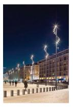
The luminaires are equipped with 90 Watt or 140 Watt Cosmopolis lamps and arranged spirally around the upper sections of the poles in different sized groups.
